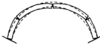
FIG. 11. Collapse mechanism for arch.
